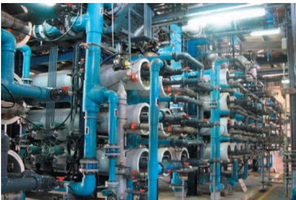
SWRO membrane process
