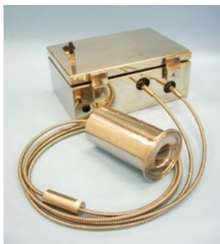
Figure 6 Spectroscopic analyzer and diffuse reflection detecting probe (approx. 65 mm in diameter)
