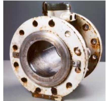
Admag lasted more than 5 years in a digester blow line where other meters lasted 6 months.
