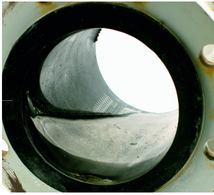
Photo A: Example of liner wear at low velocities. Because of Admag's retained liner design, this meter continued to function.
