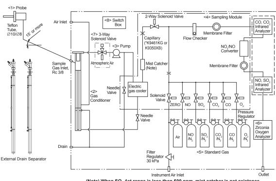
Example 2: Five Gas Components Gas Sampling System Configuration
