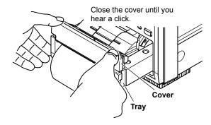
7. Push the printer unit (push the area to the left of the lever on the front panel) back into the WT1800 until you hear a click.
