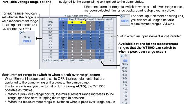
is set to OFF, the measurement range increases in the order specified by the measurement ranges whose check boxes have been selected.
