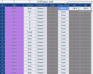
Select the mode of the D/A output range (Fix, Manual).
