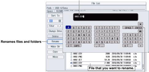
Press **ENTER** on the keyboard or the **ENTER** soft key to confirm the entered name.
