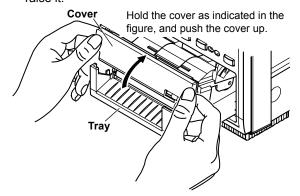
**5.** Pull approximately 10 cm of the roll paper out, and load the roll paper in the holder so that the thermal side of the paper is facing up. Load the paper so that it passes through the guides.
