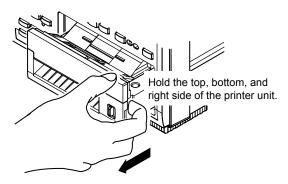
**2.** Insert your finger into the groove on the right side of the printer unit.
