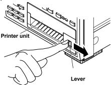
3. Hold the top, bottom, and right side of the printer unit, and then pull it toward you until it stops (pull the unit approximately 5 cm).
