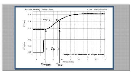
As shown in the strip charts below, begin by identifying the time at which the measured process variable first reacts to the change in controller output – not the time when the controller output first changes. In the example shown, the measured process variable shows a distinct change beginning at approximately 4.1 minutes.
