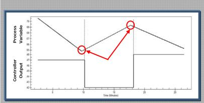
The first example shows a trend depicting a series of changes to valve position and their associated impact. The data was taken directly from the plant's data historian. As the arrows point out, the data suggests that the process variable started to change before the valve's position was adjusted. That is either a sign of a very smart and psychic process or one where the data doesn't adequately tell the story.
