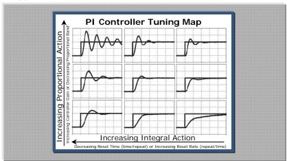
Control Station recommends use of the Internal Model Control (IMC) tuning correlations for PID controllers. These are an extension of the popular *lambda* tuning correlations and include the added sophistication of directly accounting for dead-time in the tuning computations. The IMC method allows practitioners to adjust a single value – the closed loop time constant – and customize control for the associated application requirements.
