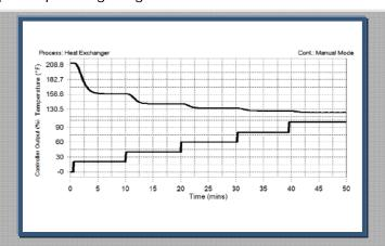
The plot shown above depicts the nonlinear dynamics of a simple Heat Exchanger process. Notice how the controller output is stepped five (5) times in equal amounts of 20% but the response of the process variables changes dramatically from the first to the last change.
