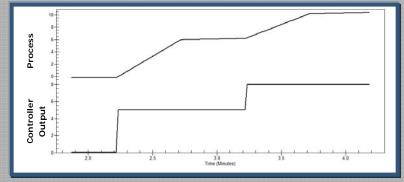
The second example involves a flow loop where data was collected at a rate of 30 seconds. When trying to assess the dynamic behavior of a process, it is important to have access to data that is collected fast enough so that the shape of the response is visible. In this case, data from the plant's historian only shows the starting and ending points associated with the increases to controller output. Absent is any truly useful information related to the process' dynamic behavior.
